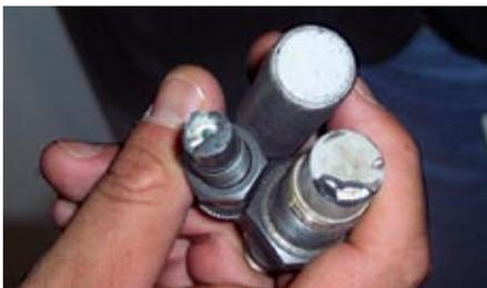
*These sensors have been destroyed by impact or abrasion. One-piece stainless steel sensors are the go-to sensors for harsh sensing environments. They can take brutal punishment and still keep functioning.*
